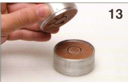
13. Place the two parts of the mould together. Replace the vertical marks in the same position. The mould is ready for casting.
