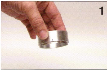
1. Place ring on a flat surface with the raised rim down.
