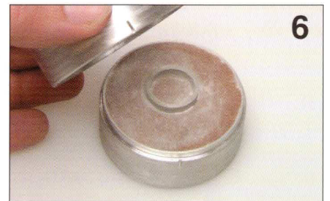
6. Place the second ring on the filled ring with the vertical marks on the two halves aligned.
