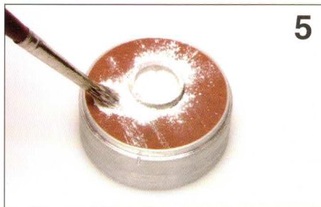
5. Sprinkle the clay filled ring with talcum powder. Brush the talcum powder over the surface.
